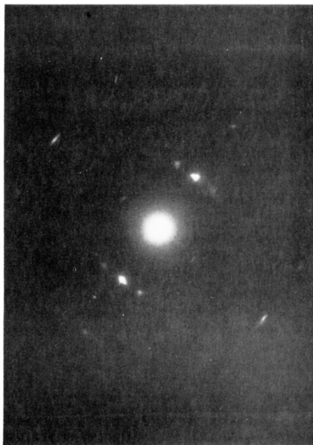
Figure 5. Room temperature electron diffraction pattern of PHBA sample ( \overline{DP} = 15 ) heated to 310 °C, held for 100 min at 310 °C, and rapidly air cooled.
